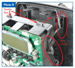
Step 16: For the *Ozotech EOG Unit* reconnect the control valve power supply to the wall outlet. Connect the EOG power supply cord to power supply jack and plug the EOG into the wall outlet. Skip to Step 17 if using *Nelsen Unit* with optional integrated power supply cord.
