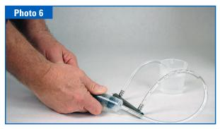
Step 6: Once the cell has been completely flushed and the water is clear, it's time to dry the cell. Use a compressed gas duster (or computer dust spray) by placing the nozzle into one of the barbs on the cell and depressing the trigger until the moisture is gone from the cell, Photo 7.
