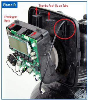
Step 6: If you have not already done so. Unsnap the top of the drive bracket using your thumbs and forefingers to expose the backplate. Photo E.
