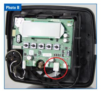
Step 4: For the *Nelsen EOG Model*, Reference 2 on previous page, disconnect the power supply from the control board, Photo C.
