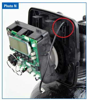
Step 12: Route the gray EOG wire through the hole along with the power supply as shown in Photo O.
