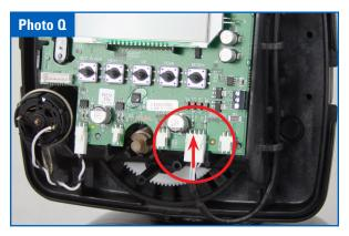
Step 15: Both the gray wire and power supply must fit into the wire chases. Snap the bracket back into place. (Do Not Press on Control Board, use the bracket to snap into place.) Photo R.
